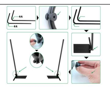
Step 2: Insert the long end of the Support Arms into the center Coupler Piece. Then slide Support Arms into the Pivot Arms.
